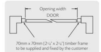
Fitting to Cardale Quick-fit steel Slideaway frame, within the brickwork aperture
