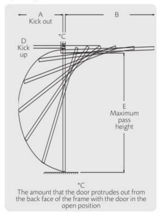
Fitting to timber frame, behind the brickwork aperture
