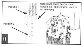
Still with the door in the open position and wearing eye protection fit lower spring anchors as shown and fit springs to spring anchors in orientation shown (See fig H).
