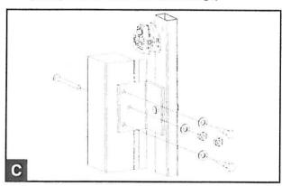
Drill pilot holes and secure each main pivot bracket in place using two M8 × 50mm coach screws and M8 washers per side. (See fig C).
