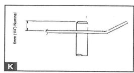
ENGAGEMENT NOTE On adjustment of top latch, please ensure a nominal 6mm (1/4") pin engagement through catch bracket (Figure K). Adjustment of all other latches should also be set to 6 mm latch overlap.
