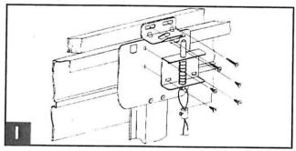
Always use both hangers on each side. For 2 springs use outer hooks, for 1 spring use centre hook, for 3 springs use all hooks. A minimum of 2 through to maximum of 6 springs per side maybe supplied depending upon door weight.
