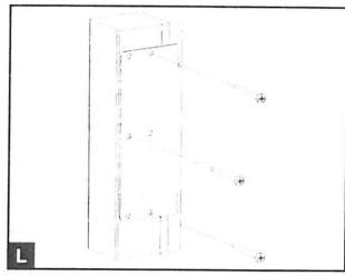
Doors over 7'6" in height (2286 mm) have an additional latch plate supplied which is secured close to ground level to provide additional wind load resistance. Align plate with the three holes prepierced in the lower side seal and secure using 3 off 6 mm x 50 mm gold self tapping screws per side (see Fig L) There is no need to pilot drill for these screws
