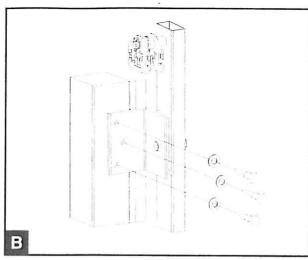
Drill pilot holes and secure each main pivot bracket using three  $M8 \times 50$ mm coach screws and M8 washers per side. (See fig B).
